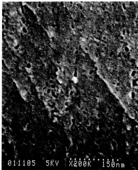
FIG. 7. SEM image of the cross-sectional structure of the sample exhibiting a large number of pores. The surface was coated with a thin Pt film.
